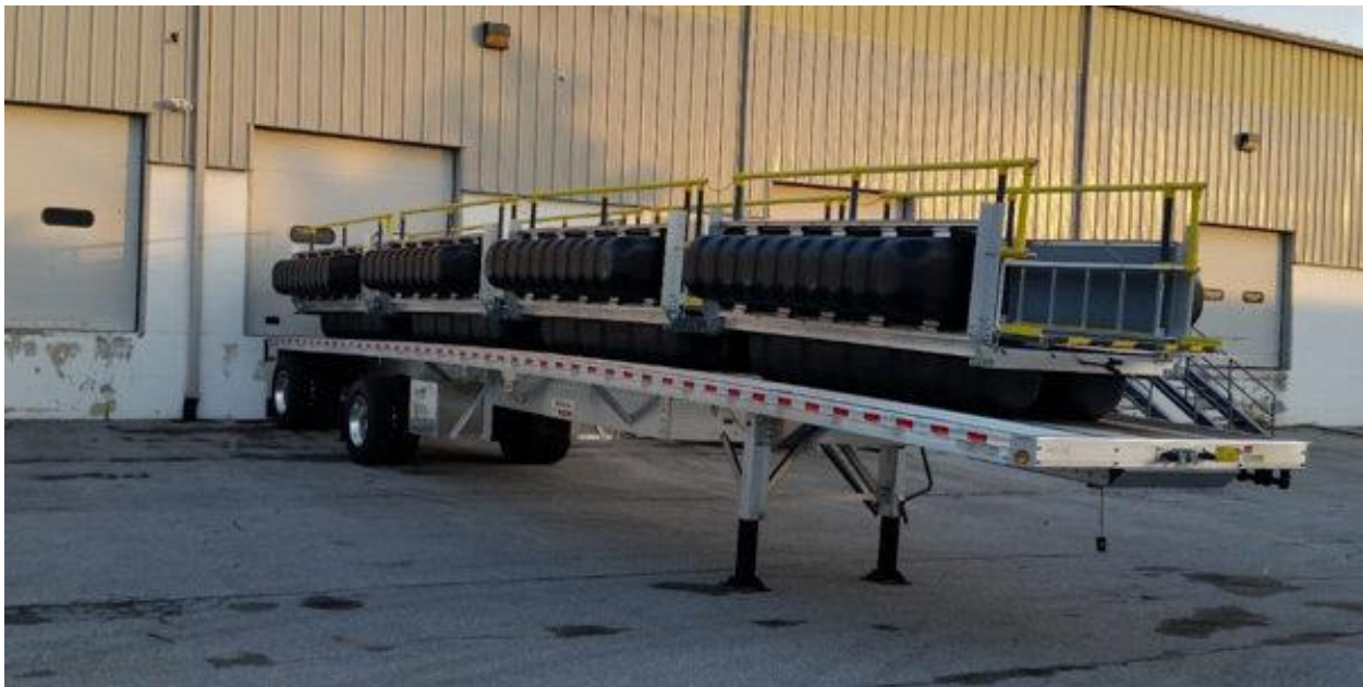
15 meter of pivot walkway with additional high buoyancy floats folded to the side
